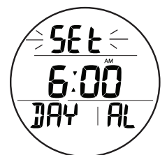
Fig. 22 - DAILY ALARM STATUS (Set, ready)
